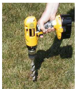
Use Soil/Wood Auger for creating 6" hole.
